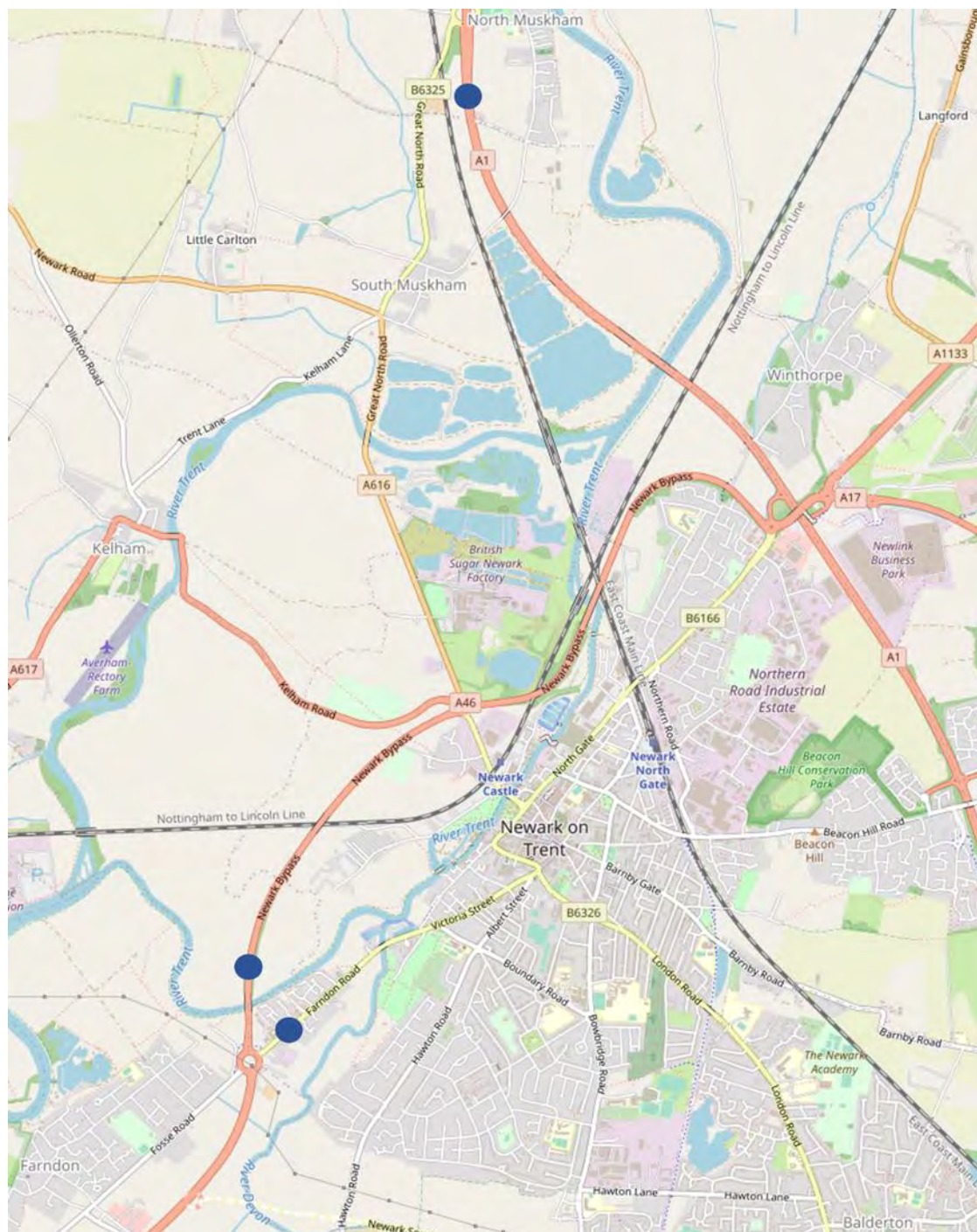
Figure 16-2: ATC locations for speed distribution calibration
